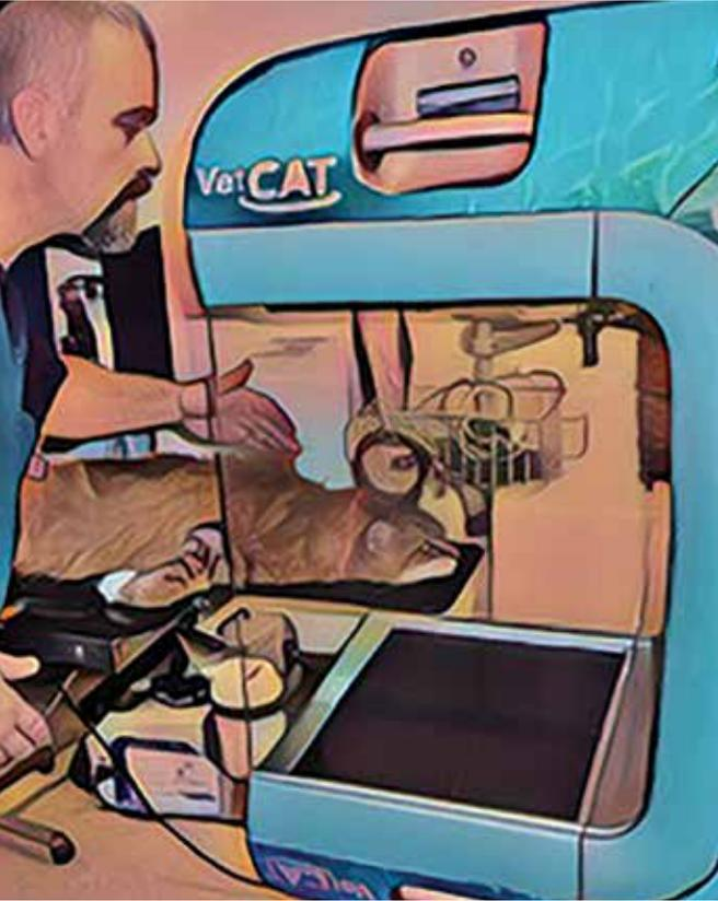
VetCAT generates high-quality, fully 3D images with submillimeter resolution and geometrical accuracy superior to multi-slice, full-body CT scanners.
